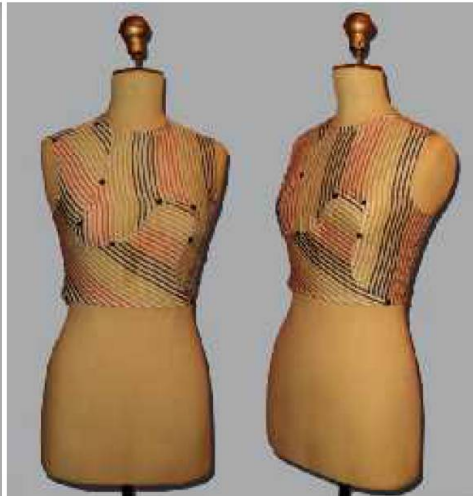
Final fitted bodice in striped fabric, using style lines instead of basic bust and waist darts
